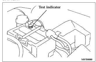
The condition of the battery is very important for quick starting and proper functioning of the vehicle's electrical system. Check the battery at regular intervals.
